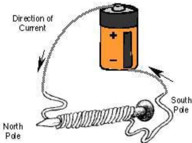
Step 6: To TEST the power of the electromagnet, attach one end of the wire to the north pole of the battery (+ end) and the other end of the wire to the South
