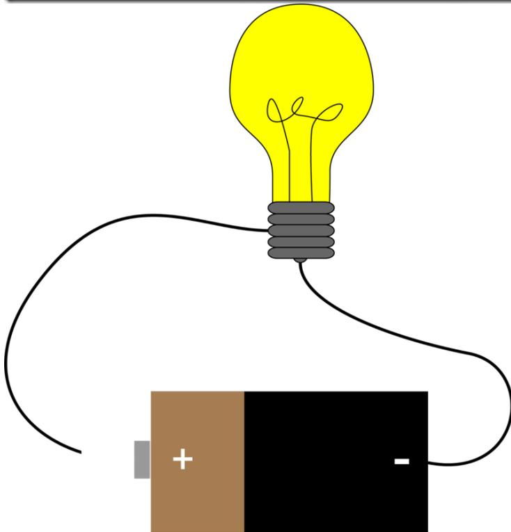
Step 3: With two aluminum foil “wires”, a D-cell battery and a light bulb, give students 5-6 minutes to see if students can figure out how to connect the parts to create a circuit which lights the power source, the light bulb.
